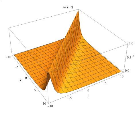
Notice that as t increases, the x-coordinate of the waveform's peak decreases. In other words, the waveform is moving in the negative x-direction.
